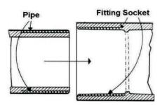
1. Area of pipe & fitting to be softened by solvent cement
