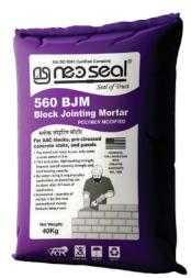
NeoSeal® 560 BJM Block Jointing Mortar is a high-strength adhesive for quick and firm laying of AAC blocks with thin joints. Made of cement, graded sand, and blended with polymers, it provides high strength and water retention properties even when in thickness of 3 mm layer against 12 to 18 mm conventional mortar.
