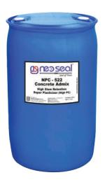
NPC - 522 (HIG PC) is the super plasticizer based on second generation polycarboxylic ether polymers, developed using nano-technology. The product has been primarily developed for applications in high performance ready-mix concrete to facilitate high early strength gains with super slump retention. NPC - 522 is free of chloride & low alkali. It is compatible with all types of cements.
