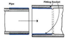
2. Apply a layer of cement in the fitting socket, and a layer of cement on the pipe. Sufficient cement should be applied for proper gap filling.
