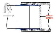
3. Assemble the pipe and fitting while the surface is wet. Rotate the pipe up to ¼ turn, and push in to the socket until it reaches to the bottom of the socket.
